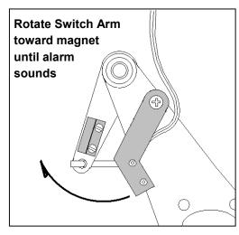
Hold switch arm firmly in position with right hand and tighten lock-nut in this position using hex key provided.
