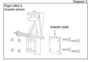
**3.** Attach SM2-2 brackets (with installed adapter plates) to mounting plates using 1/4-20 bolts and lock washers as illustrated in Diagram 3.
